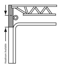
2" Track <u>Headroom:</u> 12" Radius= 11½" Required 15" Radius= 15½" Required <u>Sideroom:</u> 4½" Required <u>Backroom:</u> Door height +23" Required
